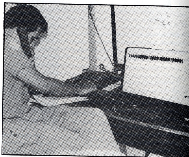
This is the new electronic switchboard being operated by Cpl Wodl and the additional switchboard for the few lines which are to be connected by hand.
